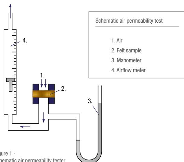
Figure 1 - schematic air permeability tester
